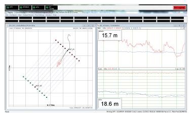
MagLogLite<sup>™</sup> Data Logging software is included with each magnetometer and allows recording and display of data and position with automatic anomaly detection. Additional software options include: MagLog Pro™, advanced logging software; MagMap™, a plotting and contouring package; and MagPick™ post-acquisition processing software.
