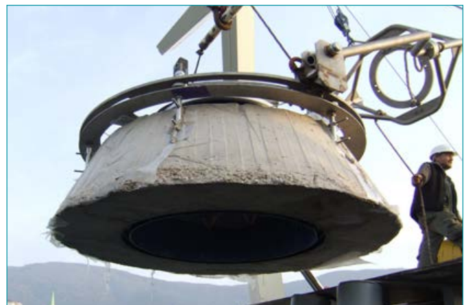
THE OPTIONAL CONCRETE DOME REDUCES NOISE AND PROTECTS AGAINST FISHING TRAWLERS
