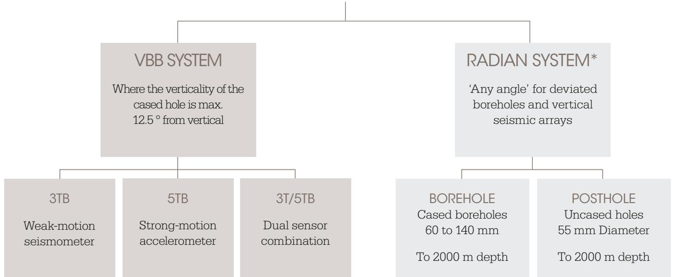
Suitable for a borehole casing diameter of 99 - 203 mm. The depth that can be achieved with the VBB borehole system will depend upon the conditions of the borehole itself e.g. Temperature
