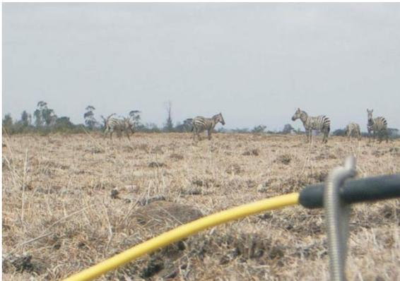
Site with AGI electrode cable and electrode stake with spring
