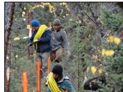
Deploying 84 electrodes in sections of 14 requires no tree cutting for minimal impact during exploration
