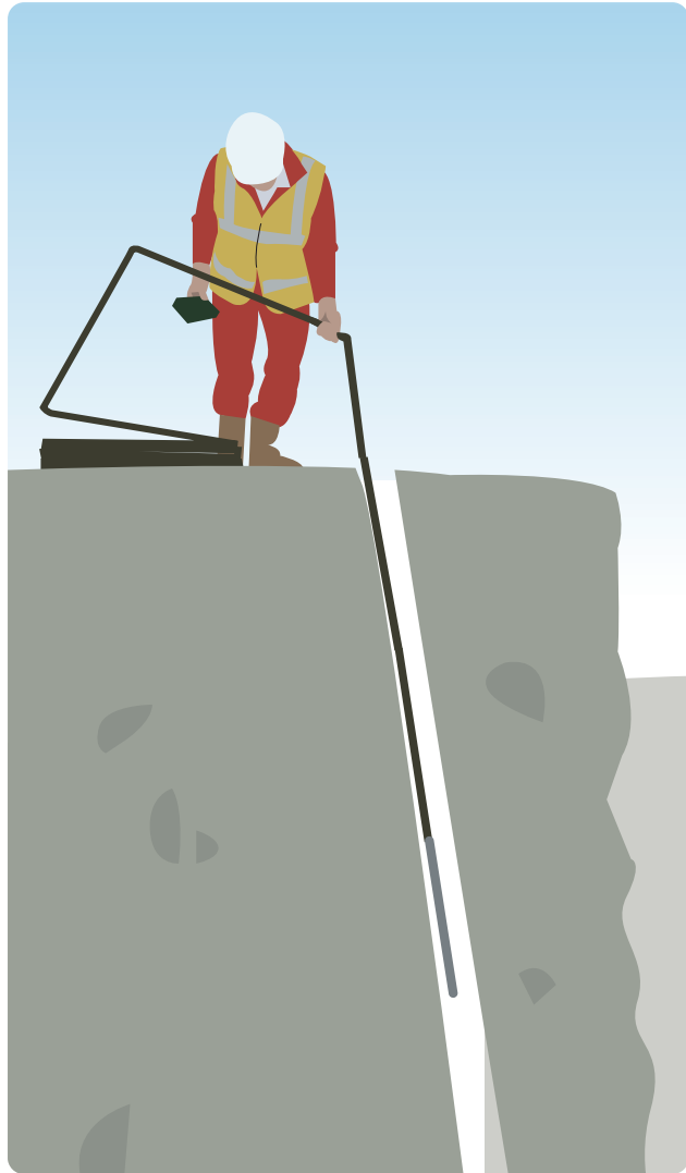
Rodded Boretrak ® being lowered down borehole
