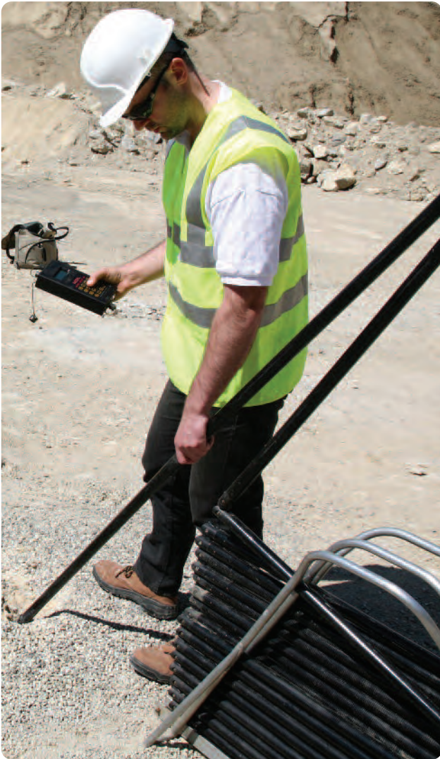
Rodded Boretrak ® showing complete system including rods and CDU logger
