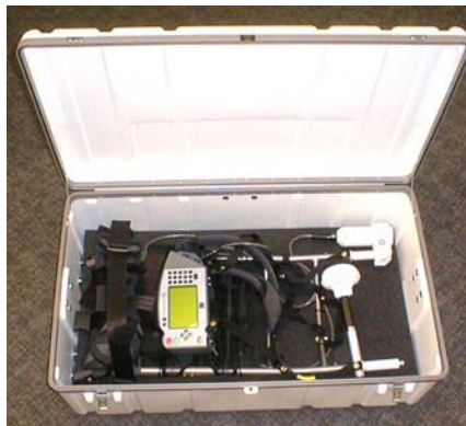
G-859 and GPS Re-Usable Shipping Case with foam padding and transport wheels
