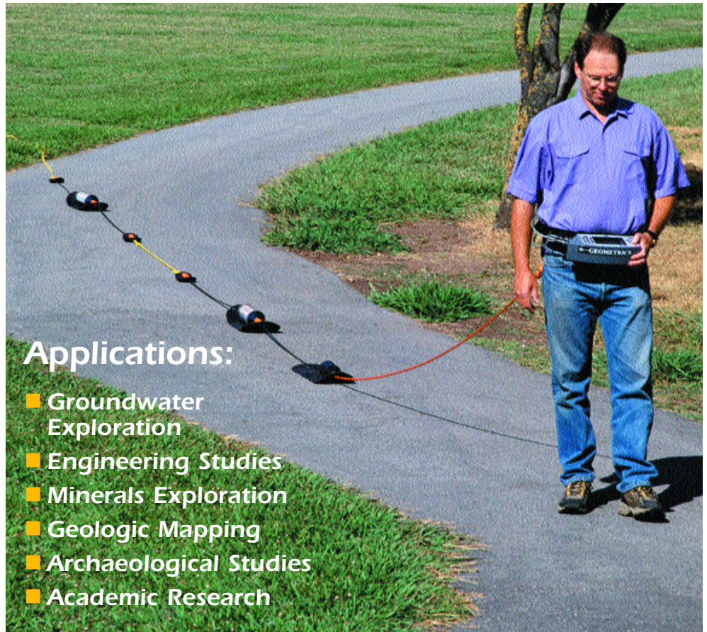
OhmMapper being towed over grass and pavement. Contact is made capacitively with the ground through insulated cables.
