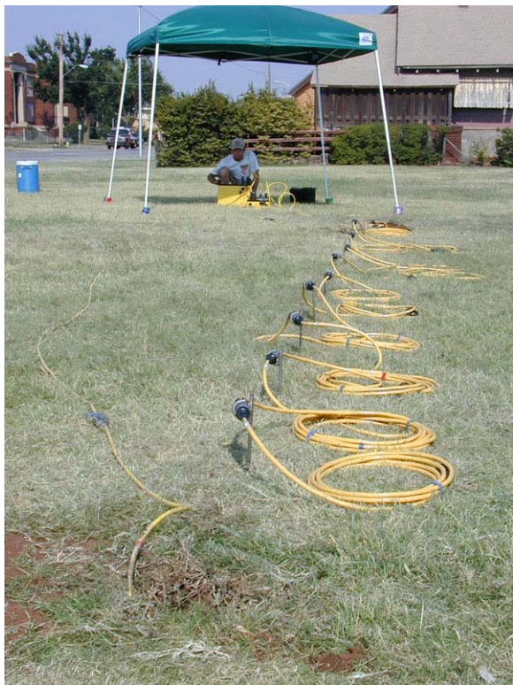
Figure 8 Surveying between two boreholes. Using surface electrodes improves the resolution near the surface.
