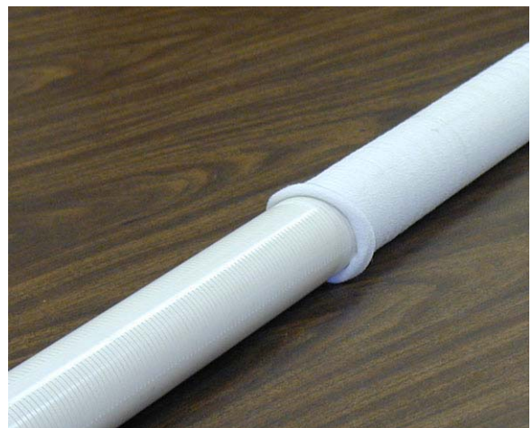
Figure 7 Slotted PVC screen. A cloth sock can be used in case small particles need to be prevented from entering the well.
