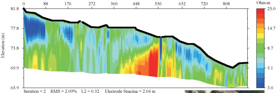
Resistivity Imaging was performed along TX State Highway 47 west of College Station, TX. The goal was to map the subsurface in this area. This area is known to have a highly variable near-surface ranging from clay to sand deposits that can be troubling during road expansion and road maintenance planning.
