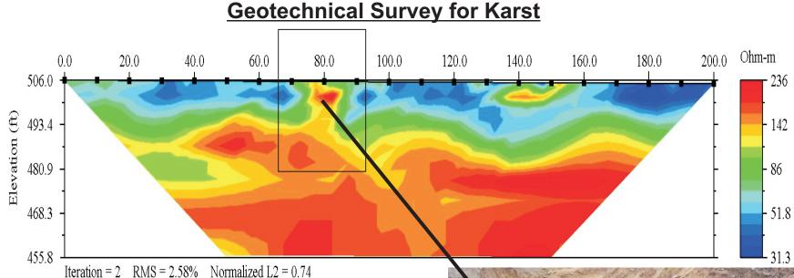
After collecting the profile shown above, the highlighted resistivity anomaly was excavated. The results of this excavation are seen in the picture to the right.
